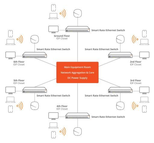
Figure 4: AON and Smart Rate Ethernet architecture
