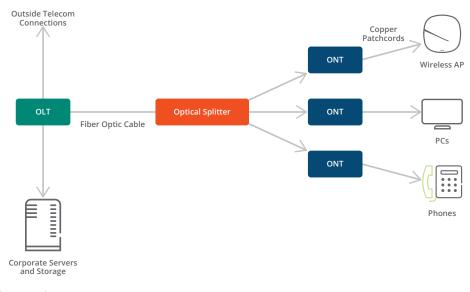
Figure 2: Basic GPON architecture for FTTX
